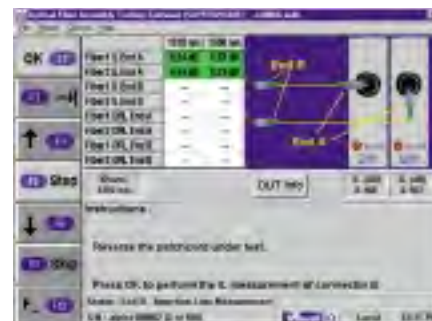
Typical setup for components under test using the IQ-12001 Optical Fiber Assembly Test System
